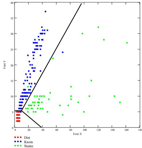
The upper left knot region can be compared to the neural network plots that will follow. It should also be noticed that one knot and one stain point are out of place and would not be classified properly by the rule classifier. These points that are out of place are called *outliners*.
