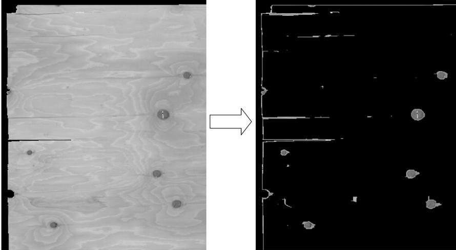
The basic idea of segmentation is to reduce the full image into areas of interest. This reduces the amount of image data that must be processed in detail. It is similar to the eye scanning process which also reduces the areas looked at.
