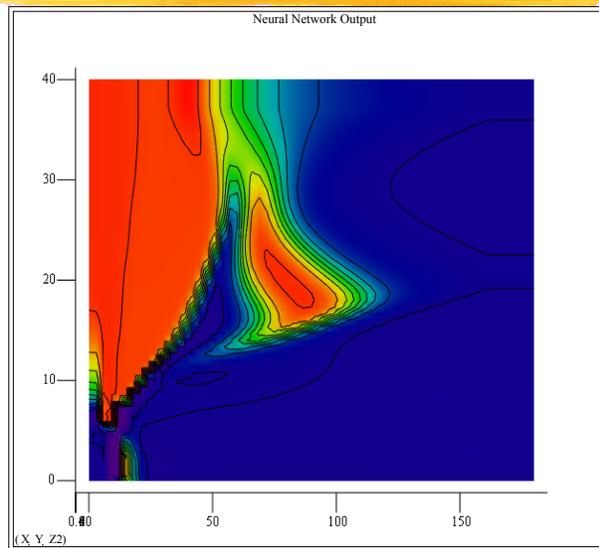
This network has two hidden layers and can fit more complex shapes. It has been able to fit a single knot point that is in the stain region.
