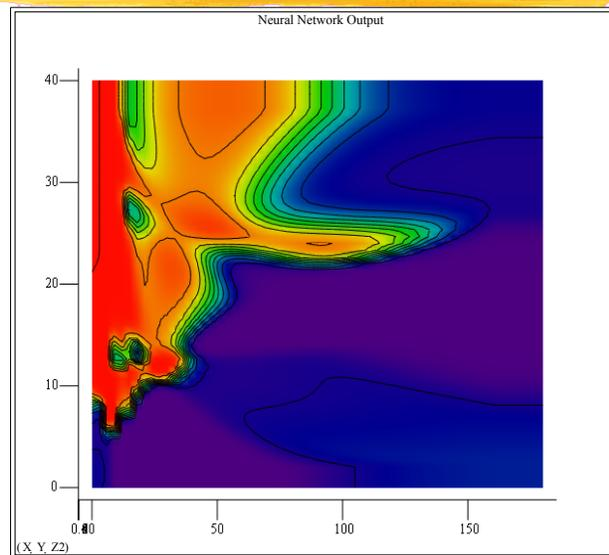
A special version of back-propagation was used to train a one hidden layer network to fit all the points. As a result of making the network fit all the points, some extra holes were introduced into the knot region.
