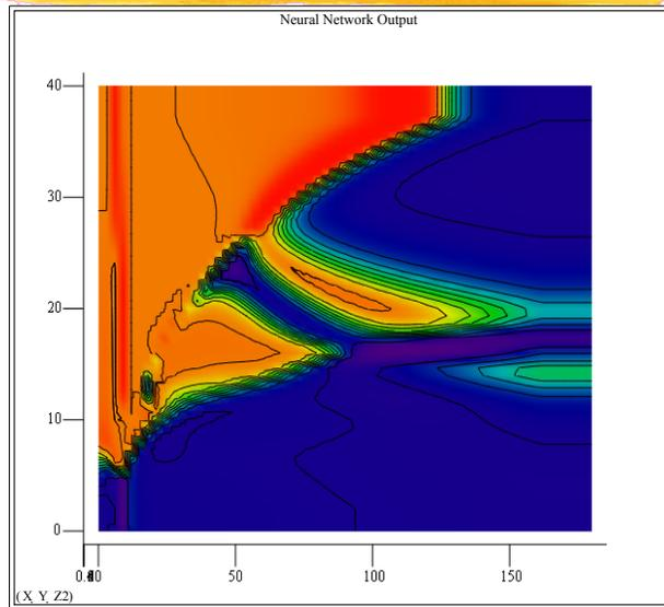
Here, the special training was used to make a two hidden layer network fit all the points. While it has fit all of the knot region correctly, it has extended large selection areas into the stain region.
